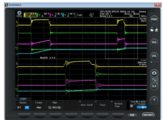
Fig.1b: Typical DPT waveforms and zoom-in
