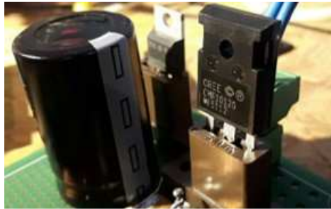
Fig. 2: Detail of the sockets for Q1 and Q2, here equipped with a TO220 diode and a CREE TO247 mosfet
