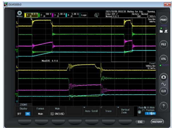
Fig. 1a: Proposed DPT topology and schematic for remote variant Fig. 1b: Typical DPT waveforms and zoom-in
