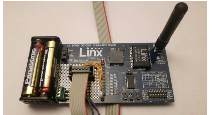
Fig. 4: Linx Rx-board with ribbon cable data connection towards a \mu Controller
